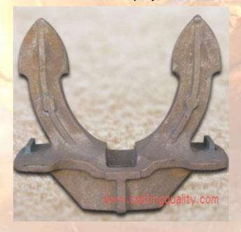
**BS3100 Gr A1 Casting Heat treatment process**: Generally all castings need to be annealed or normalized; or N+T; or OQ+T; or WQ+T
